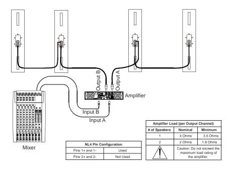
In the PSAT2 both the LF and HF drivers are connected to pins 1+/1- of the NL4 connector.
